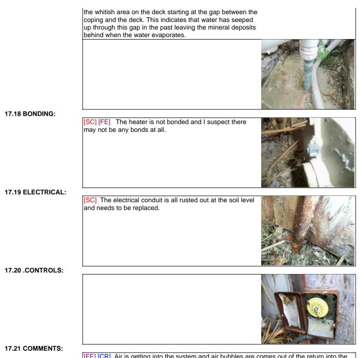
[FE] [CR] Air is getting into the system and air bubbles are comes out of the return into the pool. This continues even after the equipment has been running for a long time. Further evaluation is needed to find the source of the air intake and repair the condition. This could be easy to fix or very difficult depending on the source of the air leaking into the system.
